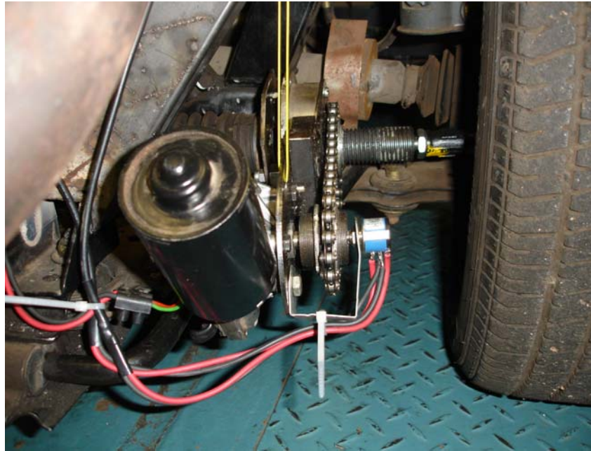
Figure 5-15: Actuator – hub assembly connection
